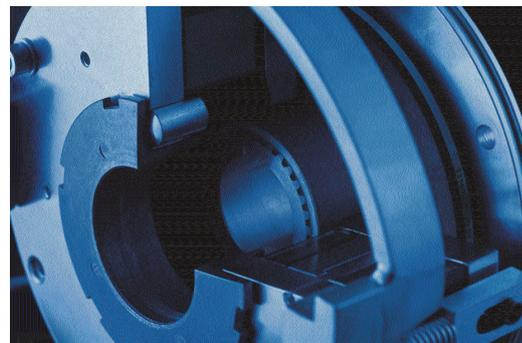
Spring applied brake designs are well-developed with high reliability and a stable friction torque that suits both dynamic braking and static holding. Standard designs with modular options are readily available with body diameters 37 to 390mm and corresponding torques from 0.1 to 2400Nm.
