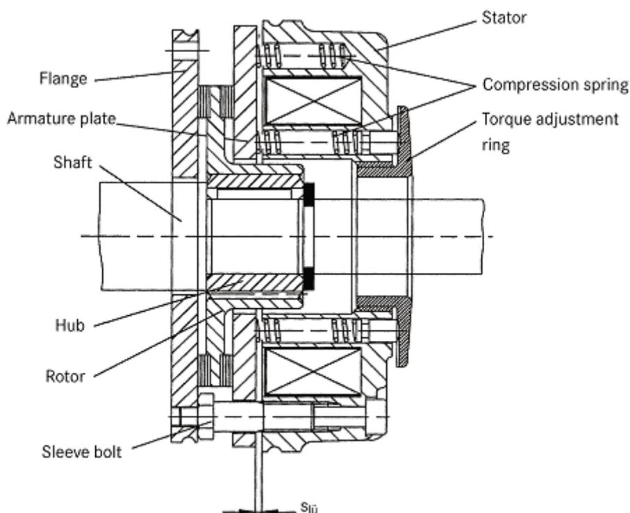
An assembly of the coil and helical springs, known as the stator, is assembled over the rotor by 3 to 6 fixing bolts. This clamps the rotor between a floating plate in the stator, the armature plate, and the machine surface. Sometimes an intermediate mounting plate is used.
